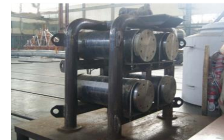
Cable Based Tsunameter (CBT)
