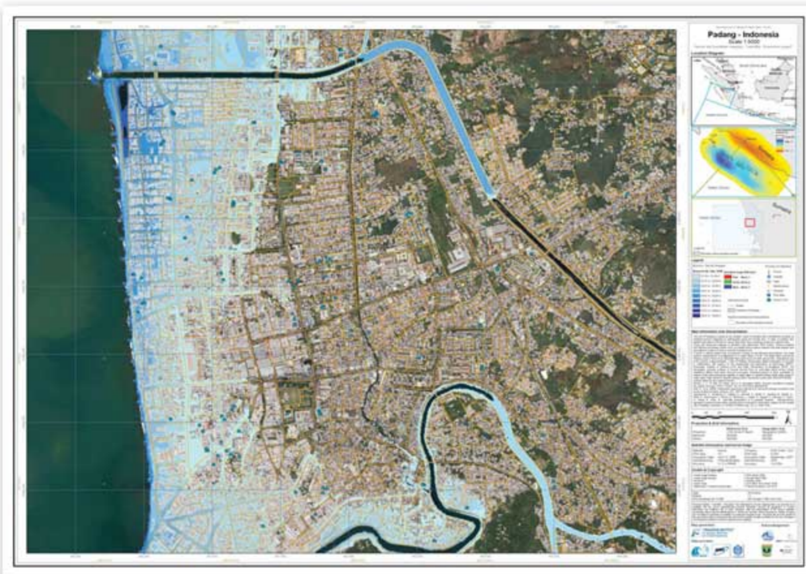
This map shows probable tsunami inundation for the centre of the City of Padang, West Sumatra, based on the most probable worst-case scenario for the area. Highly resolved topography and bathymetry data, as well as sophisticated tsunami modelling was used to produce this map (Official Tsunami Hazard Map of the City of Padang, 2010; developed by Last Mile Evacuations Project, 2010).
