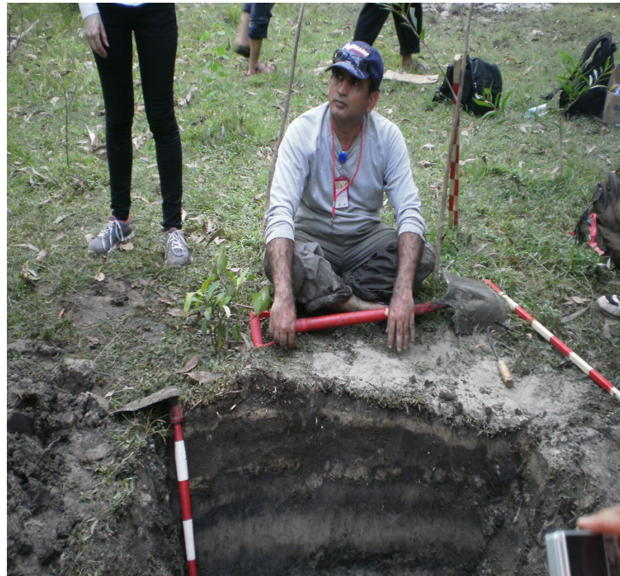
Fig 5 & 6: Dr. Brian, dewatering pit. In 2nd photo Marco taking core sampling. When the water comes into pit then we have the choice to run rotating hollow bit into ground to take core samples at different depths. Core sampling is also say lot about the subsurface, if properly place and arrange these samples on ground surface.
