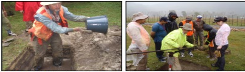
Fig 5 & 6: Dr. Brian, dewatering pit. In 2nd photo Marco taking core sampling. When the water comes into pit then we have the choice to run rotating hollow bit into ground to take core samples at different depths. Core sampling is also say lot about the subsurface, if properly place and arrange these samples on ground surface.
